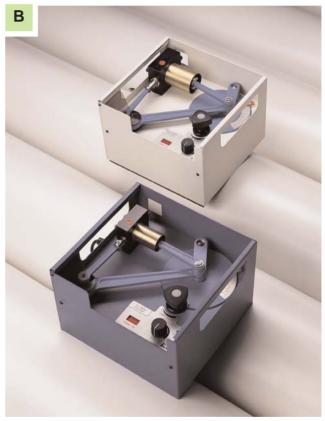
mal unrestrained for the duration of the experiment. The operator places the actuator beneath the paw (proper placement ensured via an angled mirror). A Von Frey - type filament exerts an increasing force to the plantar surface, starting below the threshold of detection and increasing until the animal removes its paw. At the retraction reflex movement when the paw is withdrawn, the 3740 registers and displays then actual force at which paw withdrawal occurred.
